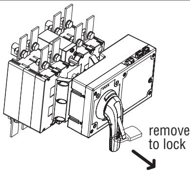
The output signal in between terminals 8 and 9 is only activated when the unit is locked via padlockable lever activation.
