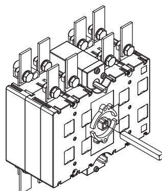
3 - Place the interface and screw it on top of the changeover switch. M5x15 DIN7985 (x6) screws and A.E.T. 5,3 (x6) washers are included.
