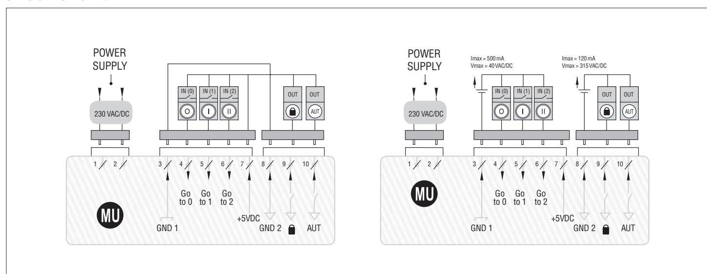
Wiring proposed for external uninterrupted supply K1, K2 = 230VAC = Coil 230VAC
