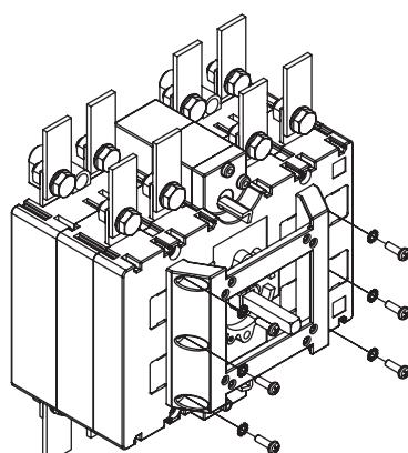
4 - Screw the motorized unit (with changeover switch and MU in 0 (OFF) position). M5 x 75 DIN 7985 (x 4) screws, A.E.T. 5,3 (x 4) washers, M5 DIN 933 (x4) nuts are included.
