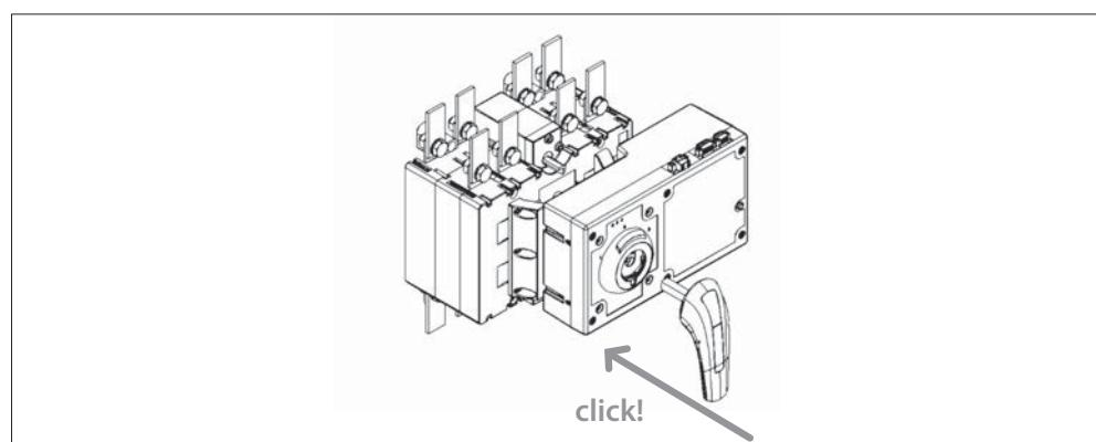
Once handle is locked the unit changes to manual operation and movements can only be performed with the auxiliary handle.
