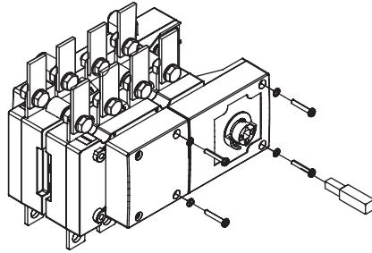
3 - Place the interface and screw it on top of the changeover switch M3.5x30 DIN7985 (x4) screws and A.E.T. 4,3 (x4) washers are included.
