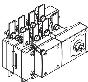
2 - Insert the coupling shaft and fix it with an allen key 2,5 DIN 90011. Without removing the front cover, remove the four screws indicated.
