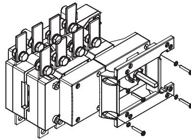
4 - Screw the motorized unit (with changeover switch and MU in 0 (OFF) position). M5 x 75 DIN 7985 (x 4) screws, A.E.T. 5,3 (x 4) washers, M5 DIN 933 (x4) nuts are included.
