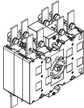
2 - Insert the coupling shaft and fix it with an allen key 2,5 DIN 90011.
