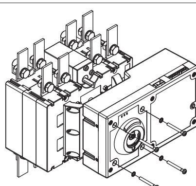
5 - Locate the connectors (CN1, CN2, CN3) and make the connections according to the electrical diagram (see annex 3, page 8).
